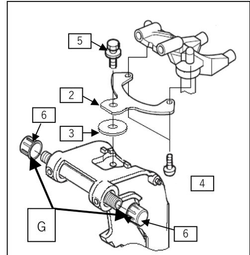
**G** : #6 cap nuts are attached to both ends of steering shaft.
