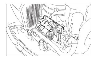
4. Open cable terminal holder cover ⑦, connect three connectors ⑧, and then close cover.
