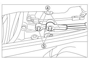
4. Adjust screw-in length of cable joint ④ so that hole of cable joint is brought to throttle arm pin and shift arm pin ⑤.
