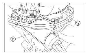
6. Install remote cont. cable stay cover ①, and then install air silencer ②.
