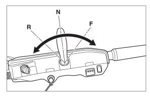
6. Check the shift lever operation.to forward (F), neutral (N) and reverse (R) position.
