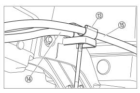
7. Install code holder (13) to multi function tiller handle, put in battery cord (14) and fuel hose (15).
