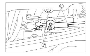
5. Lock joint with nut (6), put in on the pin, and secure with washer and R-pin (7).
