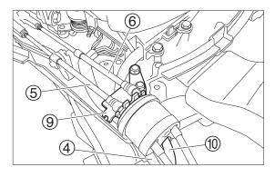
Install cable clip (9) to mount battery cable (10) and main harness (4).
