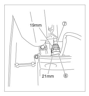
5. P (Remote steer) production model require to install neutral switch, that is included in this kit. Install neutral switch (and actuator by using wrench. (Crowfoot and U joint)
