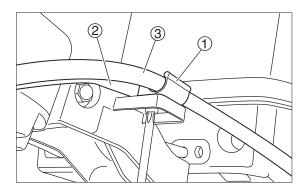
· Install cord holder ① to multi tiller handle. And then, place battery cord ② and fuel hose ③ in holder.
