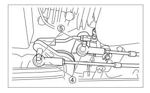
· Adjust screw in length of cable joint ④ so that hole of cable joint is brought to shift arm pin ⑤.
